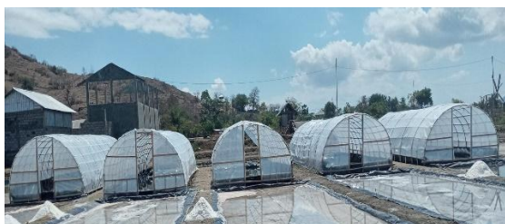
Gambar 8. Prototipe Solar House Evaporation (SHE)
