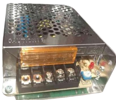
Gambar 5. Power Supply Switching
