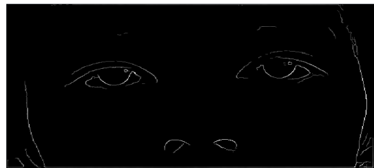
Gambar 7. Deteksi Tepi Canny
