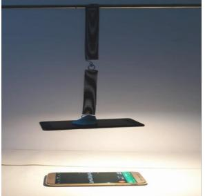
Figure 5. The photography of the serial connected spring-mass system.
