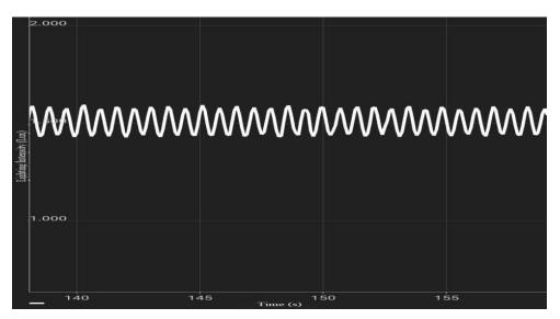
Figure 6. The oscillation screenshot of the serial connected spring system, noticeably showing the simple harmonic motion of the spring –mass system.
