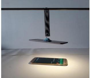
Figure 1. The photography of the basic apparatus, comprised of a spring pendulum with an oscillating smartphone as the actual mass and a stationary second smartphone.
