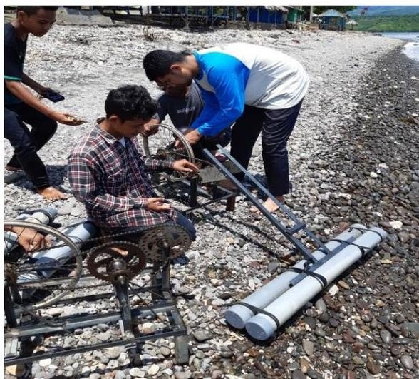
Figure 1. Testing of ocean wave energy converter prototype on the beach
