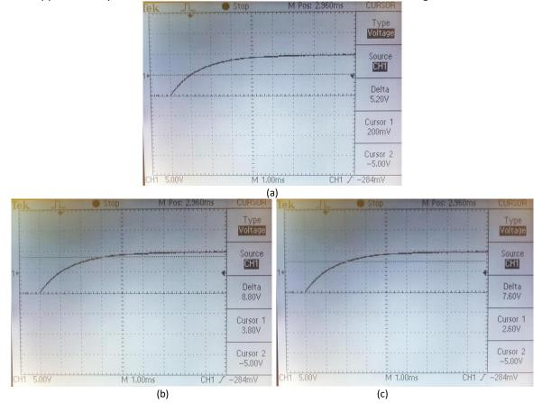
Figure 6. Experimental Voltage-Time Graphs of a Charging Capacitor at (a)  $t=\tau$ , (b)  $t=2\tau$ , and (c)  $t=3\tau$
