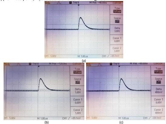
Figure 9. Voltage-Time Graph of an Inductor at (a)  $t=1\tau$ , (b)  $t=2\tau$  and (c)  $t=3\tau$
