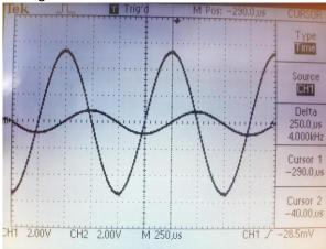
Figure 7. AC voltage-time graphs obtained experimentally are shown for the both resistor (larger amplitude) and capacitor (smaller amplitude)
