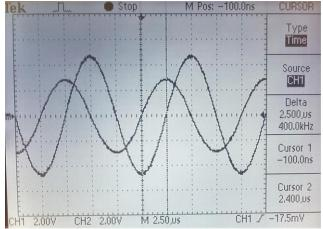
Figure 10. AC Voltage-Time Graphs Obtained Experimentally Are Shown for the Inductor (Larger Amplitude) and Resistor (Smaller Amplitude)
