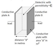
Figure 1. Structural Parameters of a Parallel Plate Capacitor
