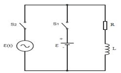
Figure 4. Circuit Employed to Resolve Both DC and AC Behaviors of Inductors
