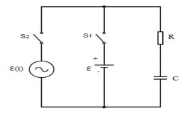
Figure 3. Circuit Employed to Resolve Both DC and AC Behaviors of Capacitors
